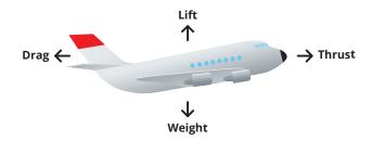
Four forces; thrust, lift, drag and weight are needed to make a plane fly.
